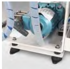
Vibration-isolation mounts reduce noise and vibration.
